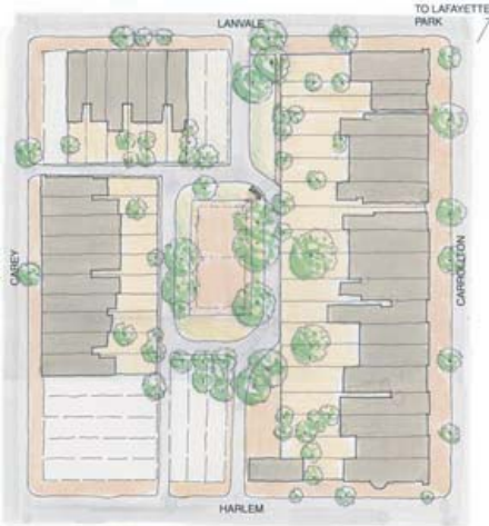
TYPICAL INNER BLOCK - 95% IMPERVIOUS PAVING
