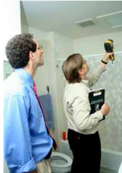
Infrared camera inspection reveals hidden energy leaks.
