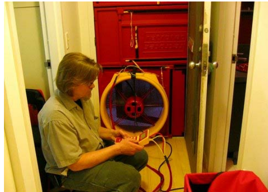
Performing a Blower Door Test (from TerraLogos files, not included in Article)
